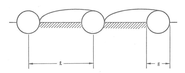
Figure 5. Cavitation model. Ellipsoidal cavity bubbles trail behind round grains. The grains are small enough that the ambient pressure several grain diameters above them is the surface pressure  $p_s$ .
